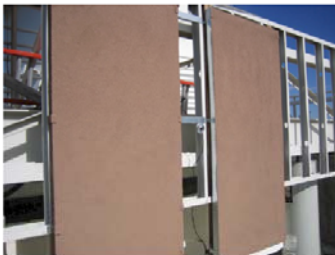
Solar thermal collectors resembling stucco during tests at the University of Nevada, Las Vegas
